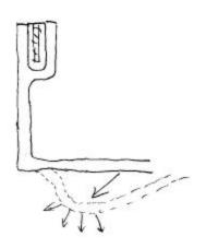
Water low in diaphragm – heel pushed upward. This can occur any time the diaphragm is under-filled. The rubber heel cannot bend out because of the can wall. The arrows show the bending force and what we see in cases like this is a crack that forms just below the radius under the metal ring.
