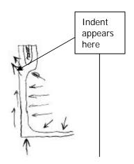
As the diaphragm is not filled properly due to a leak or rupture (fatigue crack) then the entire pressure of the ram is exerted on the heel of the diaphragm. When this occurs, the heel will collapse inwardly fatiguing the lower corner of the diaphragm. The cracked inner radius at the bottom is the result. This is normally only a result of a water deficit and will not be seen without evidence of a leak or rupture.
