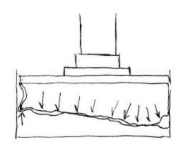
collapse. Since it is confined by the can on the outside diameter, it may collapse inwardly as shown. The collapse normally causes a "shear" failure where the cut or crack in the rubber is just under the metal ring. Alternately the diaphragm can stay vertical and try to shear off the ring. See below.
